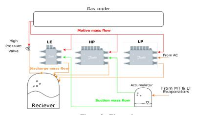
Figure 2 - Ejector layout
