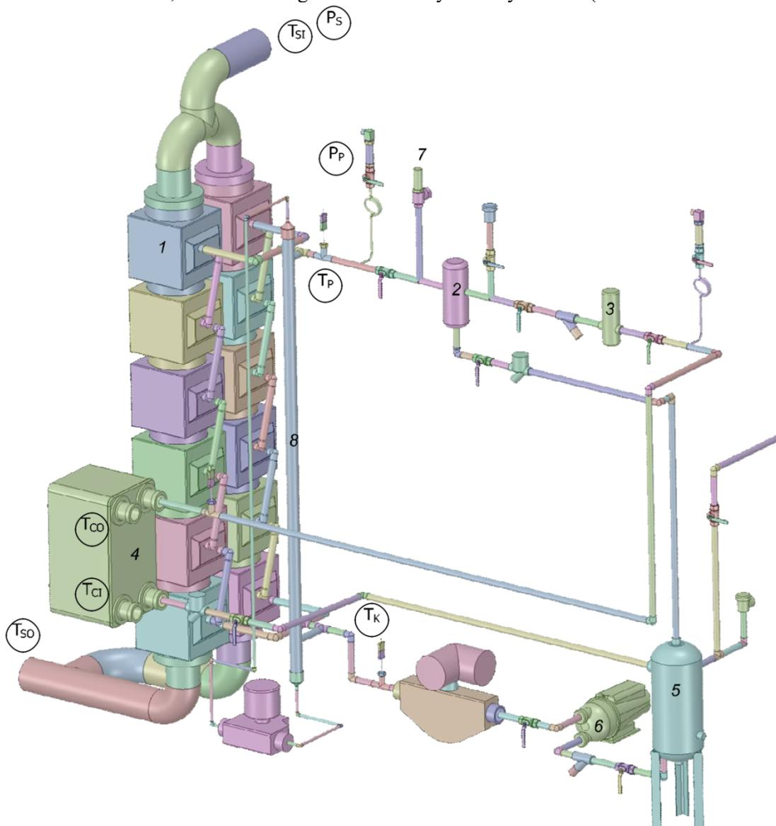
Fig. 6. Spatial schematic of the prototype steam heat recovery system: 1- section of the flue gases heat exchangers; 2 – liquid-vapour separator; 3 – pressure reduction station; 4 – steam condenser; 5 – condensate collector; 6 – pump; 7 – security valve.
