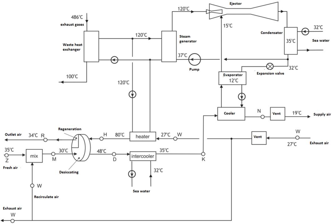
Fig. 3. Air conditioning cycle with latent heat absorption in desiccant wheel
