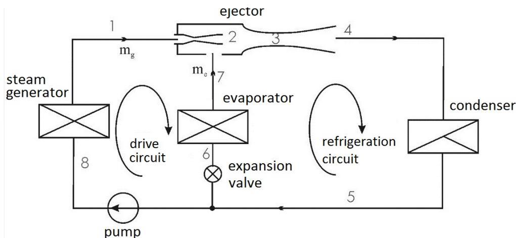
Fig. 1. Schematic diagram of ejector refrigeration system
