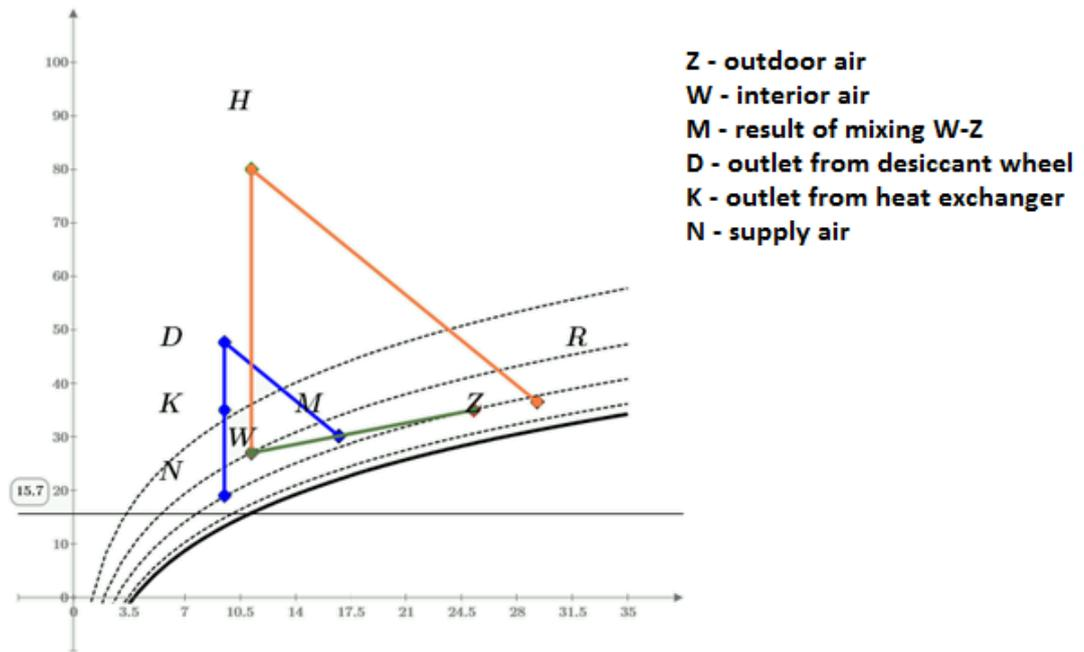
Fig. 4. Air conditioning cycle with latent heat absorption in desiccant wheel for assumed operating parameters
