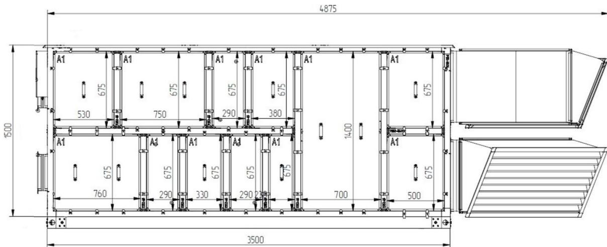
Fig. 5. View of the air-conditioning unit prepared for motor yacht.
