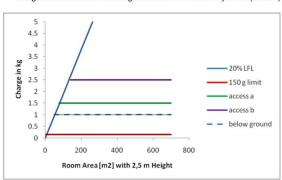
Fig.2 Examples of charge limitation for direct systems according to EN 378-1
