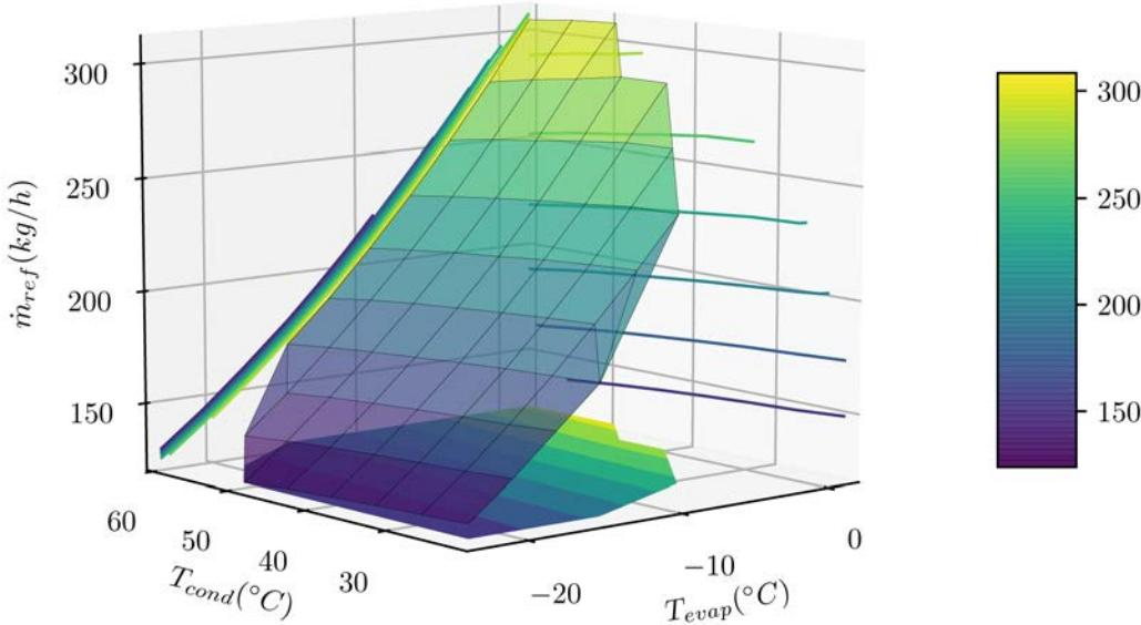
**Figure 2: 3D plot of mass flowrate versus evaporation and condensation temperatures of compressor ZS21KAE-PFV with refrigerant R404A (SH=11 K).**
