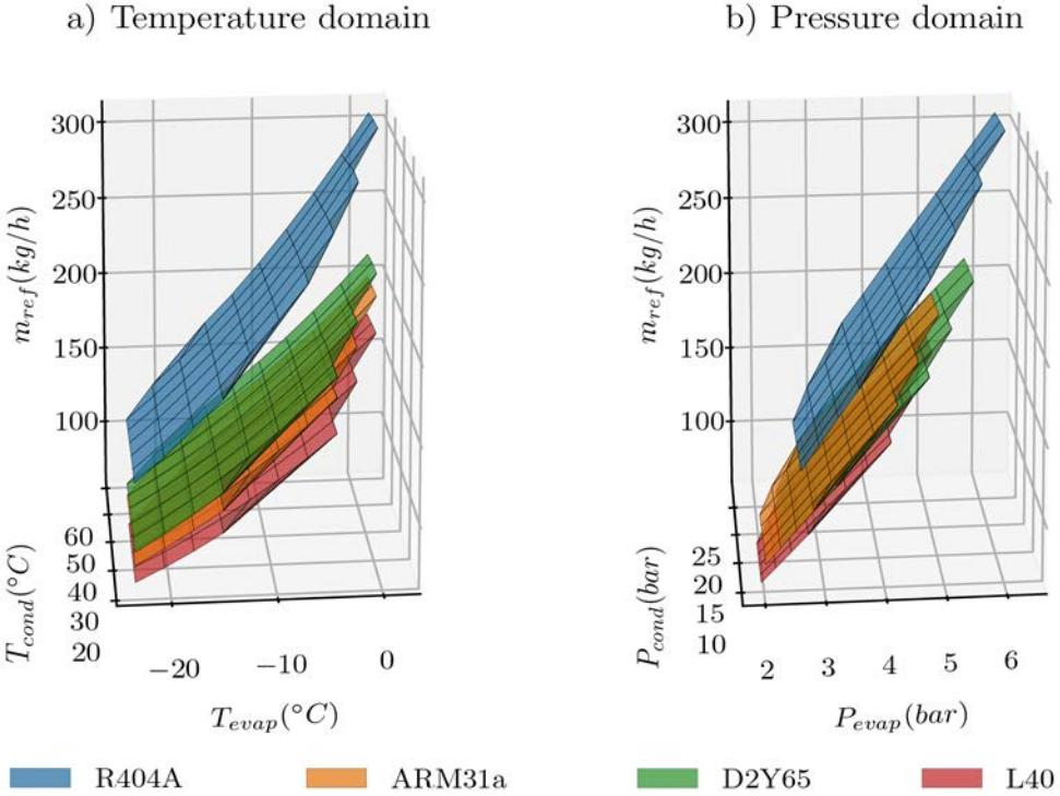
**Figure 3:** Left side: 3D plot of mass flowrate versus evaporation and condensation temperatures of compressor ZS21KAE-PFV for 4 different refrigerants. Right side: 3D plot of mass flowrate versus evaporation and condensation pressures of compressor ZS21KAE-PFV for 4 different refrigerants (SH=11 K).
