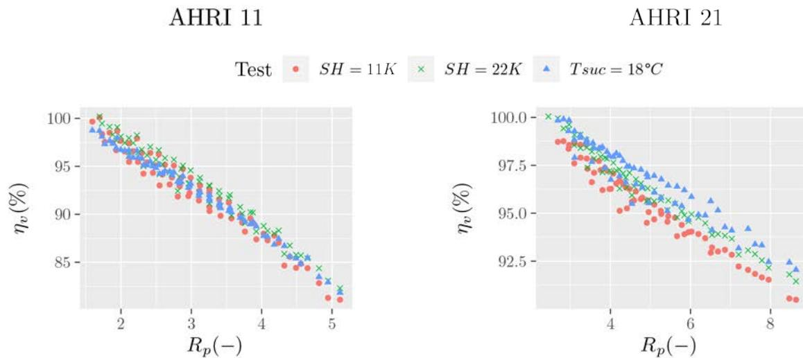
**Figure 1: Volumetric efficiency versus pressure ratio of compressors ZP21K5E-PFV (AHRI-11) and ZS21KAE-PFV (AHRI-21) for their corresponding reference refrigerant, R410A and R404A**
