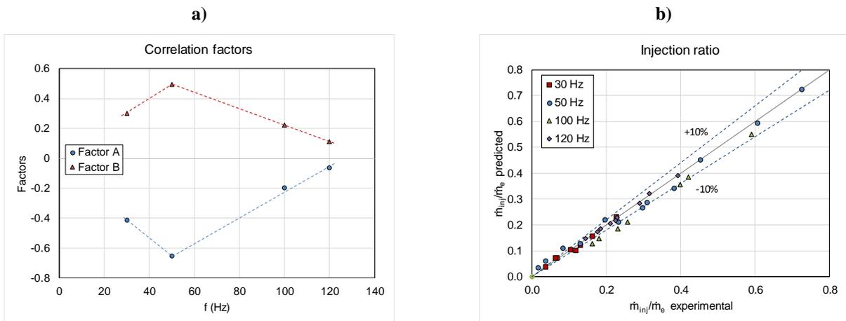
**Figure 7: a) Slope and intercept dependence on frequencies. b) Comparison of the experimental and predicted injection mass flow ratio for a VS-SCVI working with R-290.**
