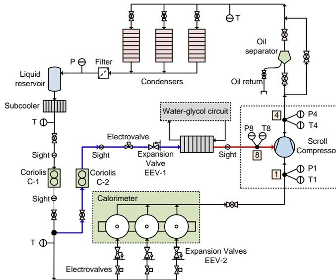
**Figure 2: Scheme of the calorimetric test bench.**
