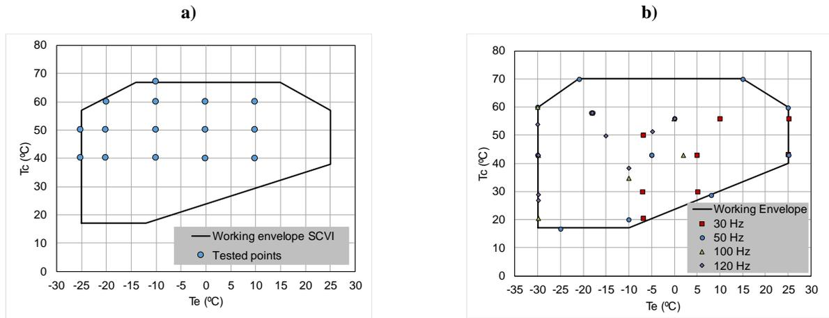
**Figure 3: Working envelope and tested points of the compressors. a) SCVI. b) VS-SCVI.**
