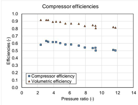
**Figure 4: Compressor efficiency and volumetric efficiency of the SCVI as a function of pressure ratio.**
