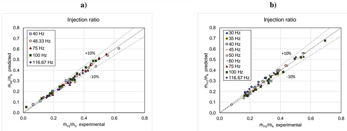
**Figure 8: Comparison of the experimental and predicted injection mass flow ratio. a) VS-SCVI working with R-410A from Dardenne et al. (2015). b) VS-SCVI working with R-410A from Dechesne et al. (2019).**
