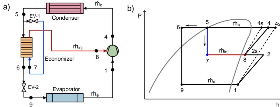
**Figure 1: Vapor injection cycle with economizer of the SCVI. a) Schematic of the cycle. b) P-h diagram.**
