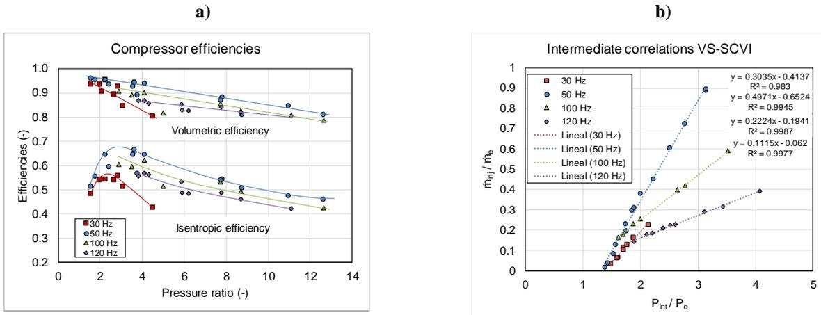
**Figure 6: a) Compressor efficiencies of the VS-SCVI as a function of pressure ratio at several frequencies. b) Injection mass flow rate correlation at different frequencies.**
