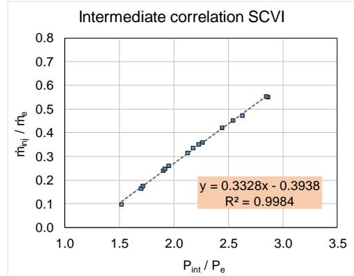
**Figure 5: Injection ratio ( $\dot{m}_{inj}/\dot{m}_e$ ) as a function of the intermediate pressure ratio ( $P_{int}/P_e$ ).**
