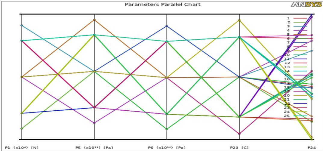
Figure 5: Parallel chart showing the variation of 4 factors and the output variation of roundness
