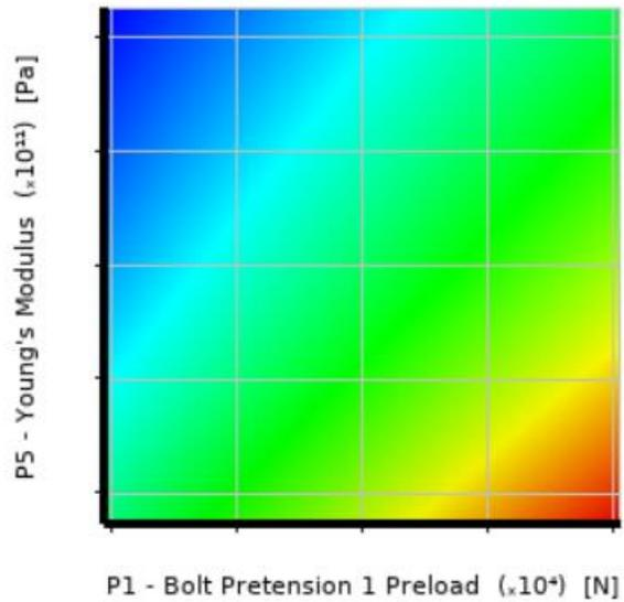
Figure 6: 2d countour plot of roundness vs. bolt pretension and crankcase Young modulus
