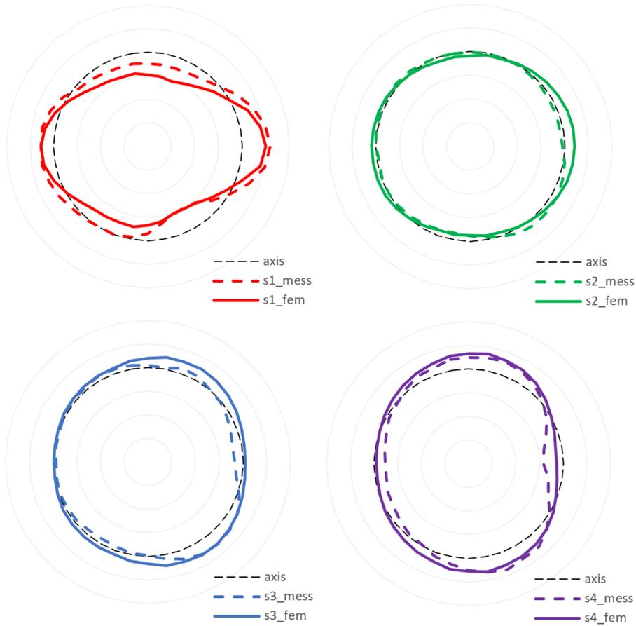
**Figure 4: Roundness plot comparing experimental measurements and numerical results by sections**
