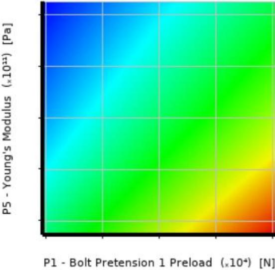
Figure 6: 2d countour plot of roundness vs. bolt pretension and crankcase Young modulus
