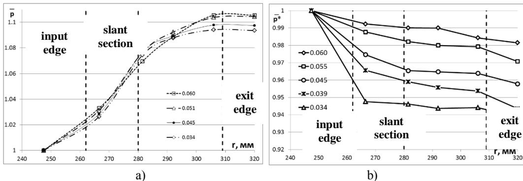
**Figure 6: The distributions of relative static pressures (a) and relative total pressures (b) on the middle line along the radius CD at different values of the flow rate  $\Phi_0$ .**
