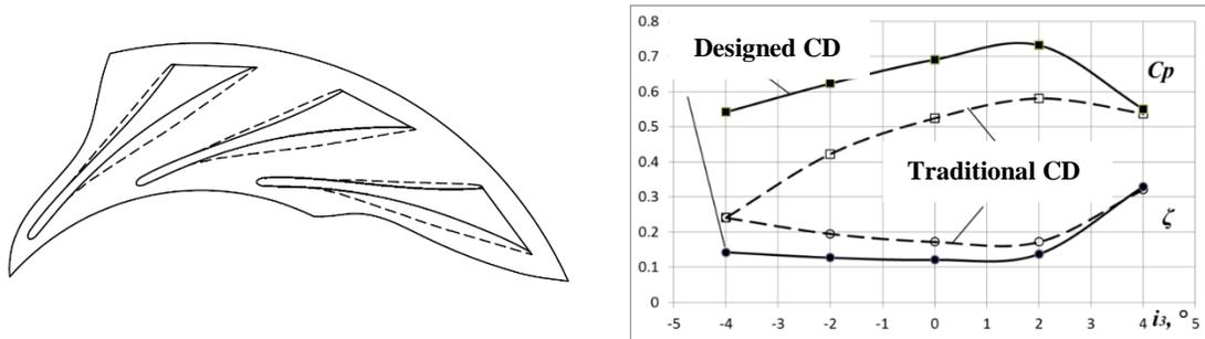
**Figure 3: Profiles and characteristics of traditional geometry CD (dashed line) and designed using the above method (solid line)**
