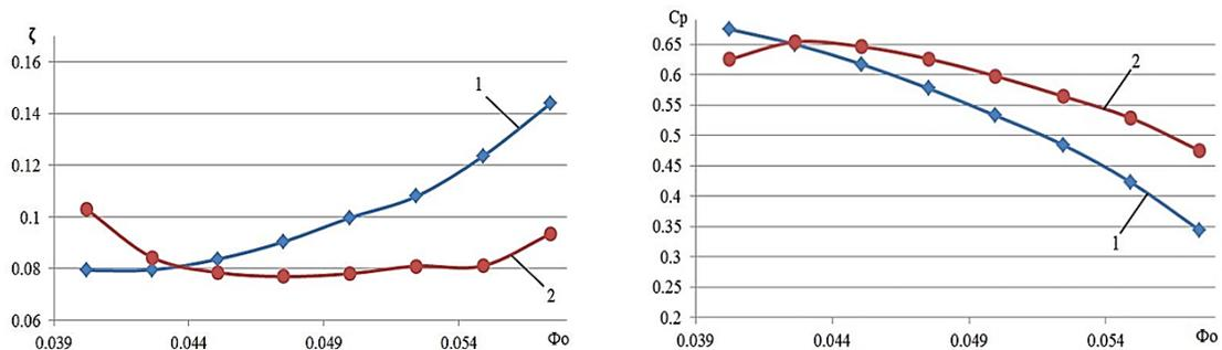
**Figure 2: Dependences of loss coefficients and static pressure rise coefficients on flow coefficient; 1—the middle line of the vane is an arc of a circle; 2—given velocity distribution on the surface of the vane**
