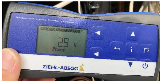
Figure 5 Measurement using Modbus protocol presented about 30 % lower fans power as multiplication of measured values as voltage, current and power factor. Using Modbus protocol next values were read as fan speed, currents, voltage, power factor, ...
