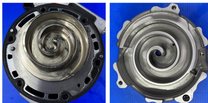
Figure 5: Disassembled scroll after compressor durability test
