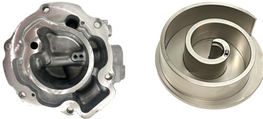
Figure 7: Compressor rear housing and orbiting scroll after teardown
