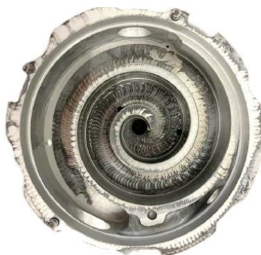
Figure 7: Compressor fixed scroll after teardown showing some deposit
